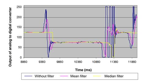
Figure 7. Filtering bouncing and joystick swings.
