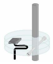
Figure 3. Mouse installation (a) Remove the handle and the protective cap of the joystick of the wheelchair, (b) insert the ring and tighten the set screw, (c) mount the protective cap and (d) reassemble the joystick of the wheelchair.
