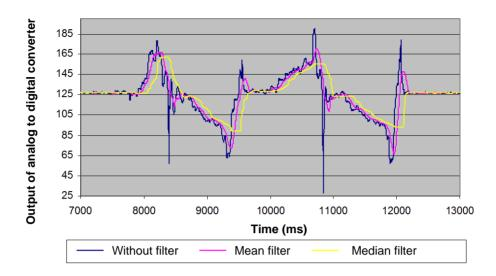
Figure 6. Effect of filtering strikes or violent actuation on the joystick.
