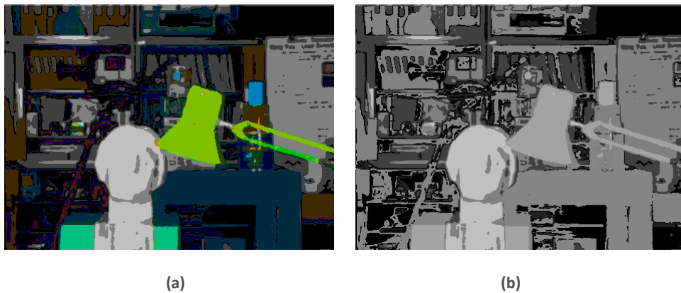
Fig. 5.36. (a) Tsukuba right image after color clustering (1 byte/pixel). False color representation. (b) PCI shown in a gray scale image.
