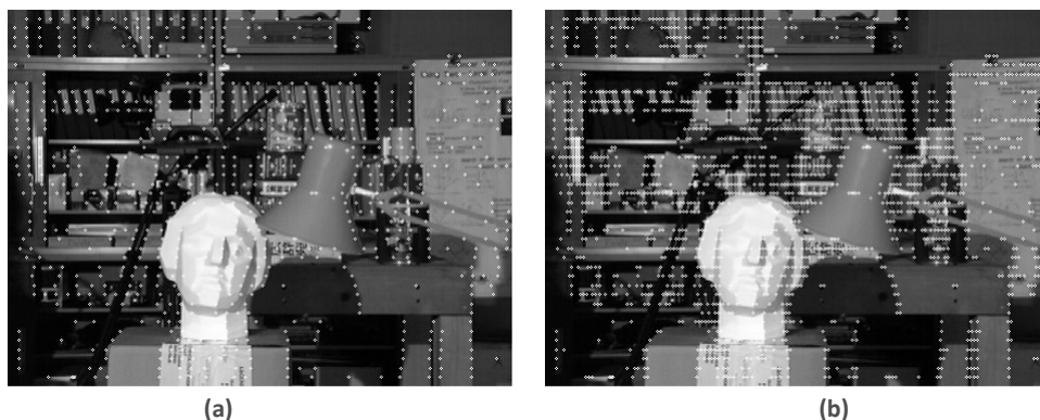
Fig. 5.41. Vertical relevant points extracted forcing a separation of (a) 9 and (b) 2 pixels. In both cases, there are 40 scan lines.
