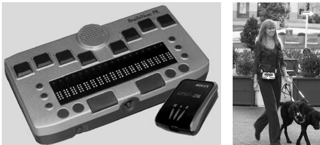
Fig. 2.33. The BrailleNote GPS, alone and being used by a blind person, from [108].
