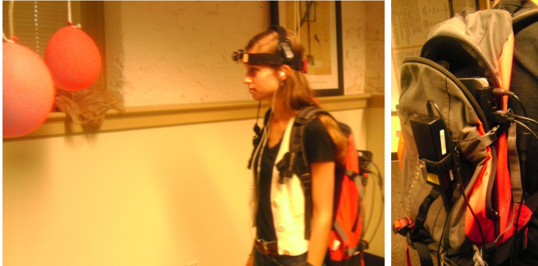
Fig. A.III.3. (left) One of the experts stands in front of the balloons, eyes opened. She wears a helmet with the webcams attached to it, the earphones and the back bag with the laptop. (Right) A detail of the back bag used to carry the laptop.
