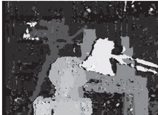
Fig. 5.27. Initial disparity map with segment regions and plane fit forcing. Image extracted from [2].
