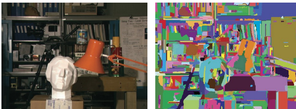
Fig. 5.26. Image segmentation of the Tsukuba pair of images. Left, original image. Right, segmented version. Taken from [2].
