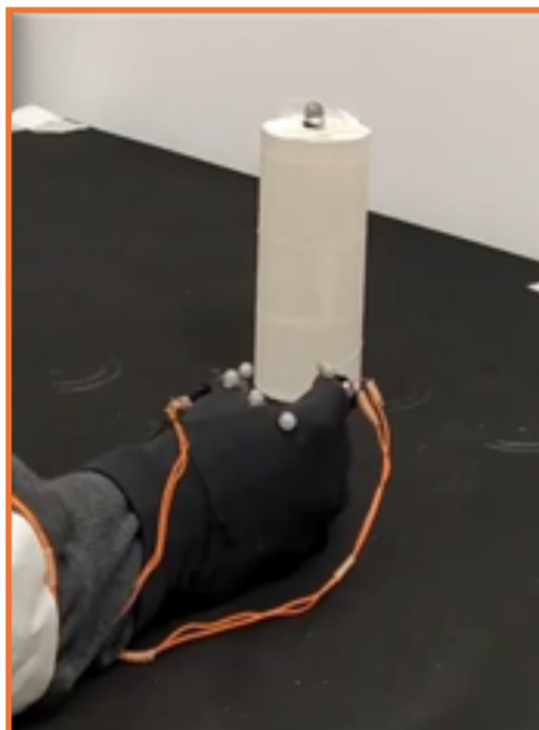
Figure 3. The SSD glove. It has 5 white reflective markers to measure the position of the hand and fingers. Two vibrotactile coin motors are positioned on the back of the index finger and thumb.
